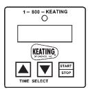
Make certain power to the timer has been OFF for at least 30 seconds. Then PRESS and hold down the UP arrow button while turning the rocker power switch to the ON position.
