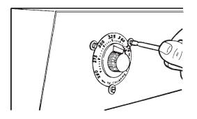
4. If calibration of griddle is found to be less than 15°F off, simply loosen three dial plate retaining screws (See Figure 4-1), rotate dial plate to match thermometer reading and tighten screws.
