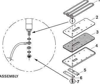
Figure 5-3 HEATING ELEMENT ASSEMBLY
