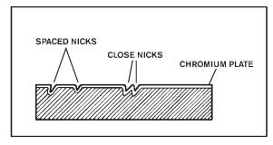
**NOTE:** Damage done to the MIRACLEAN<sup>®</sup> surface is irreparable and is not covered under Keating Warranty
