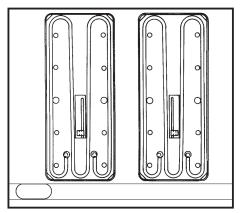
5. After each load, scrape the griddle surface completely clean using the 4" wide replaceable blade scraper.
